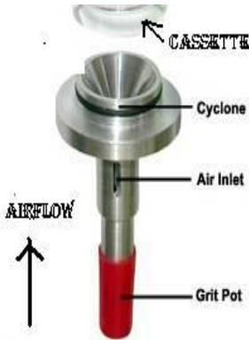
Figure 1. Recommended Silica Sampling Train
